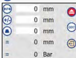
Input of the crimping dimensions, correction value and crimping dies (automatic).
