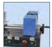
Axially adjustable clamping unit - prevents bending of small hose dimensions.
