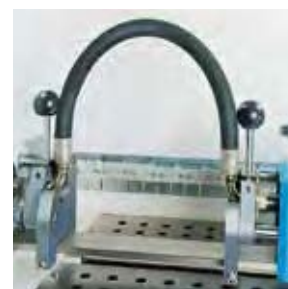
The test bench caters to a wide range of fittings and hoses.
